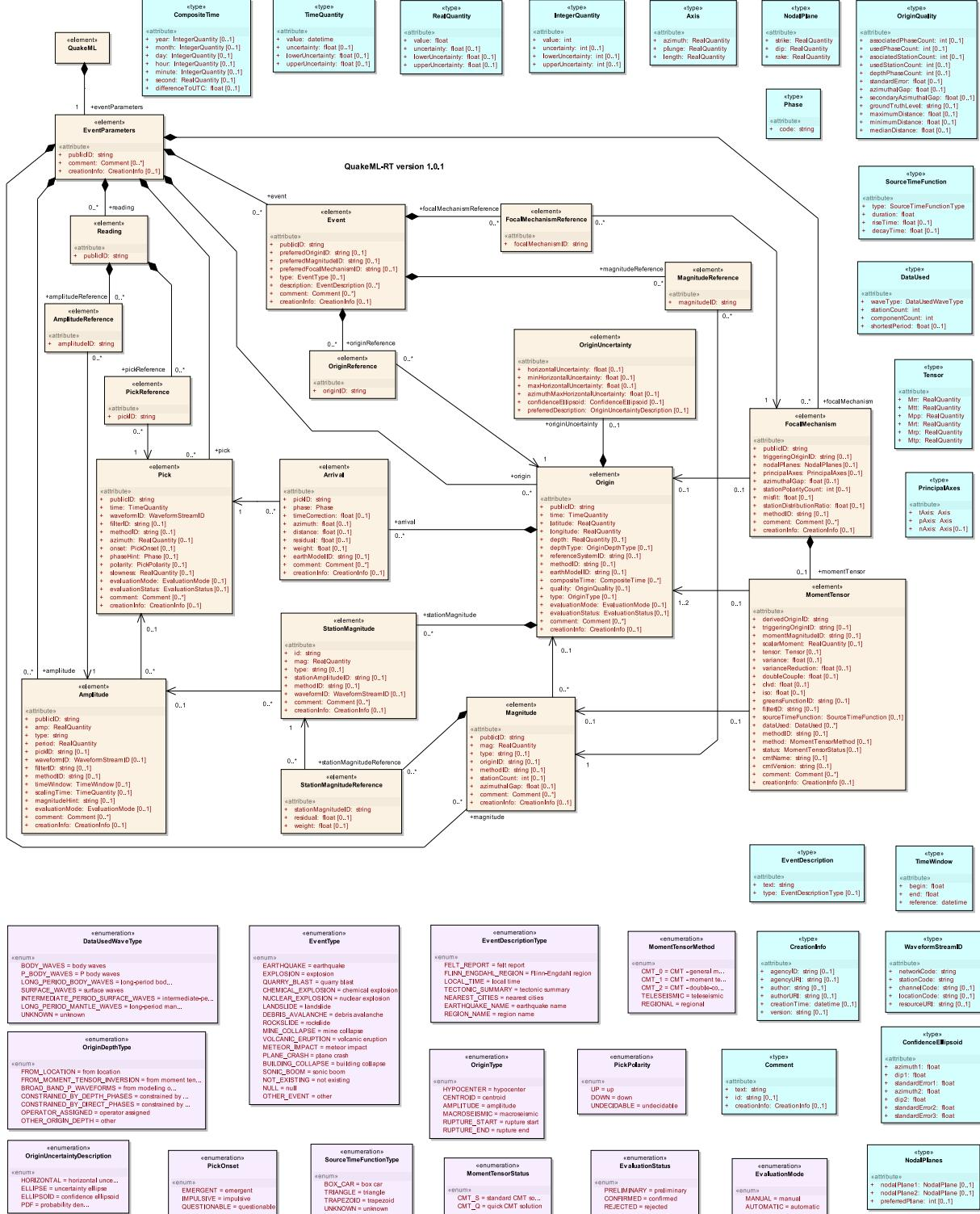
Figure 2: UML class diagram of the QuakeML-RT (real-time processing) data model.
