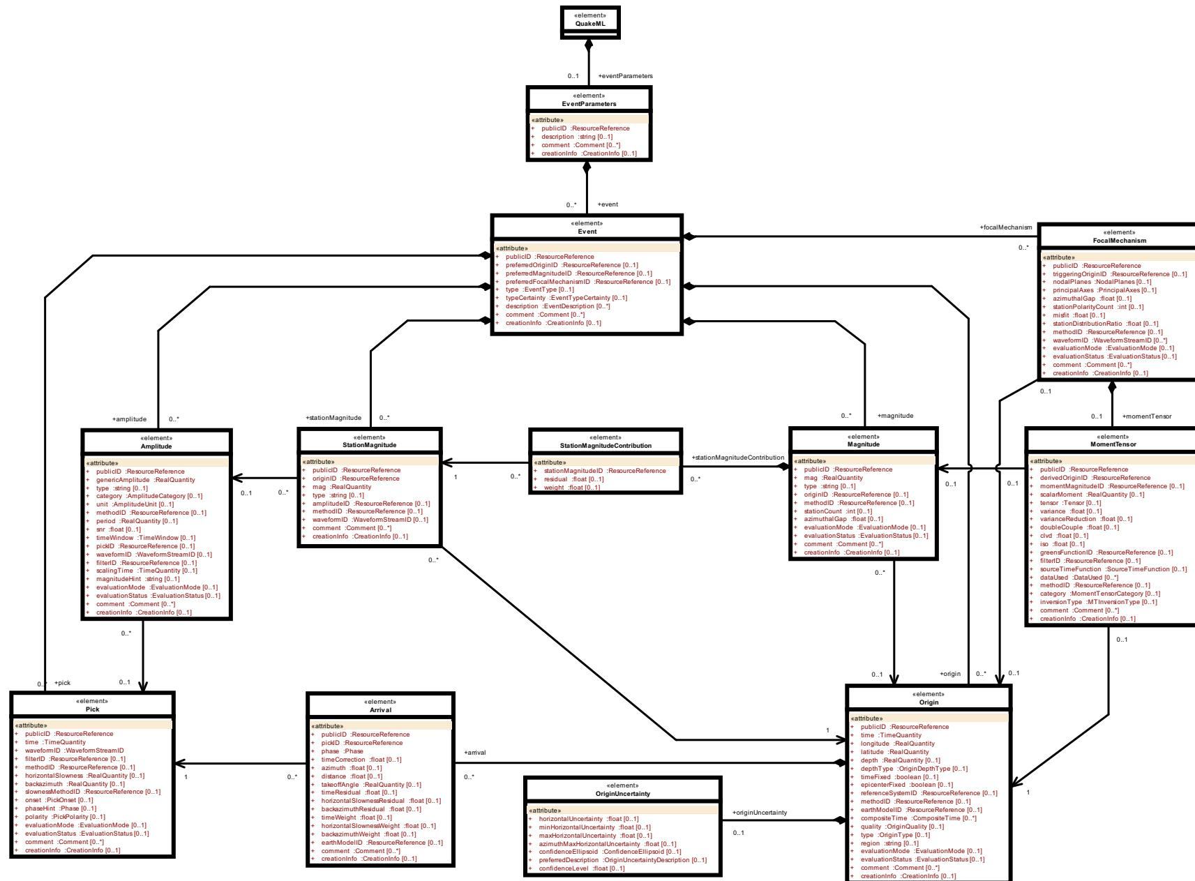
**Figure 1:** UML class diagram of the QuakeML BED data model. Two different types of relations between classes are used: (i) compositions, marked by lines with filled diamonds; and (ii) associations, marked by arrows. Compositions indicate a stronger coupling between two classes than associations.
